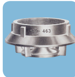
OPW-ES 463 Cast aluminum with female threads for 3" or 4" liquid loaders. Vertical wing ribs prevent drop tube from rising when filling. Accelerates discharge and prevents roiling of product when used on pressure discharge line.
